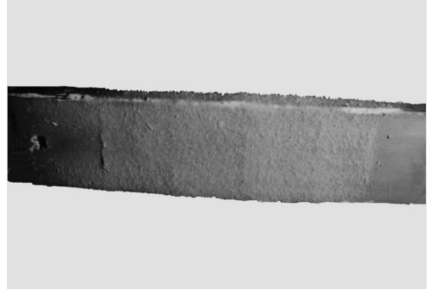
Figure 17. Heating element (surface material: stainless steel), t_e = 450 h.
